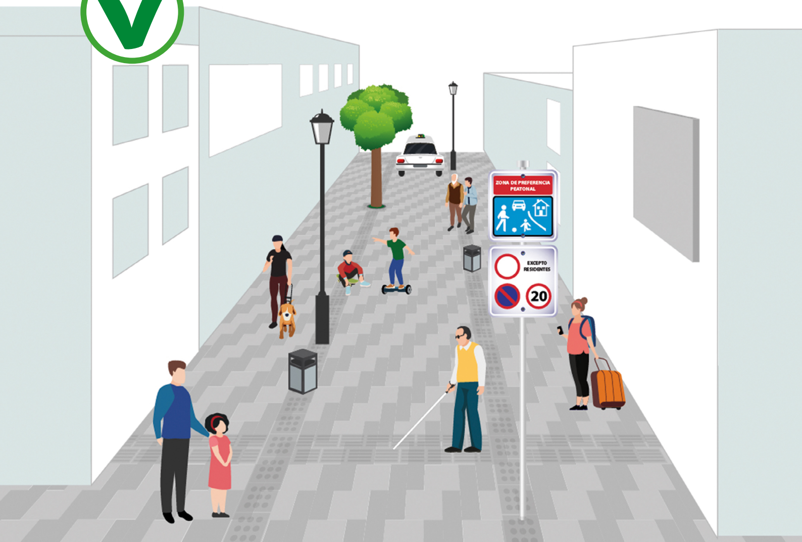
Image 20. Guidance paving connecting both safe zones.
