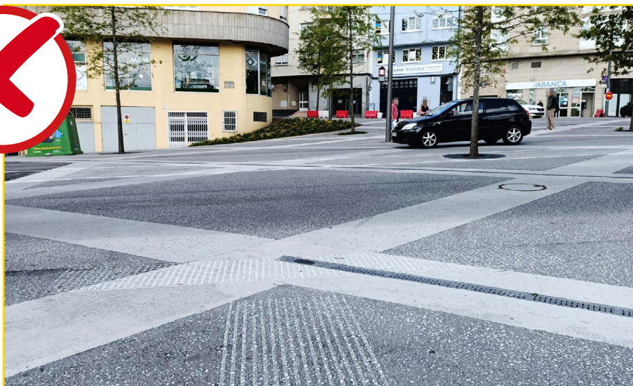
Image 32. Poor design that causes confusion between vehicular and pedestrian areas.
